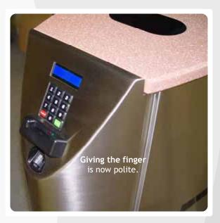
XTec offers a combination device that incorporates the three pillars of authentication: "something you have, something you know, and something you are". By combining a smart card reader, PIN keypad, and finger recognition reader into one compact unit, XTec offers a unit that prevents card lending and maximizes security.
